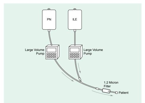
Figure 2. Setup for using a 1.2 micron in-line filter to administer dextrose-amino acids admixture with ILE given as a separate infusion.
