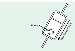
Figure 1. An example of an air-eliminating 1.2 micron in-line intravenous filter.
